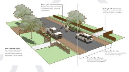
The FHWA recognizes this design as a potentially appropriate option for minor rural roads with low volumes (Average Daily Traffic or ADT<2000 vehicles/day) of traffic traveling at low speeds (<30mph) - see figure to the right.
